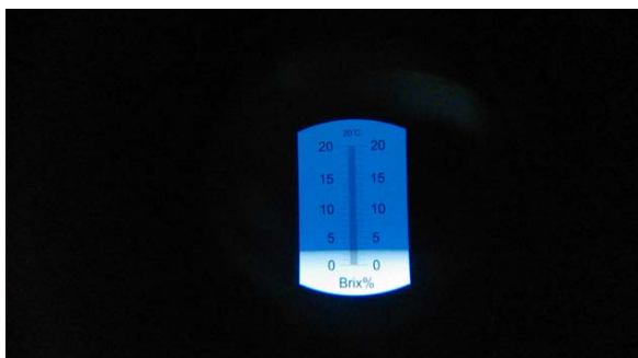
Figure 3. Refracting plate image acquired by smartphone 图 3. 手机获取的折光板图像
