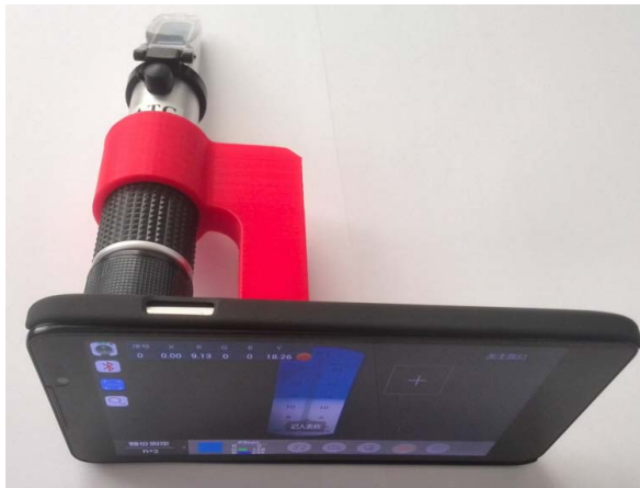
Figure 2. Visual refractometer digital device based on smartphone 图 2. 基于手机折光测量的检测装置
