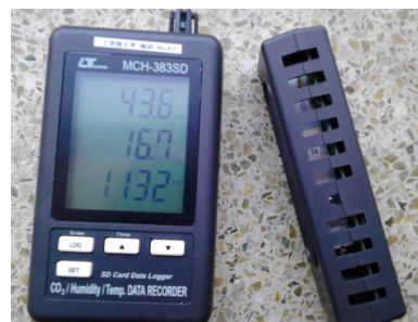
Figure 2. MCH-383SD CO 2 /Humidity/Temp Monitor 图 2. MCH-383SD CO 2 浓度/温、湿度记忆仪
