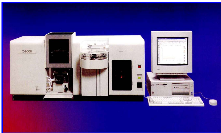
Figure 1. Z-5000 Zeeman Atomic absorption spectrophotometer 图 1. Z-5000 赛曼原子吸收分光光度计
