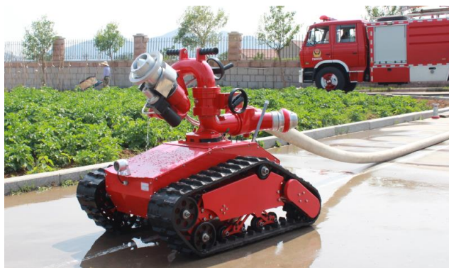
Figure 5. Near picture of fire fighting robot
