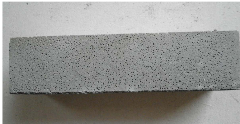
Figure 4. The air vent of the test specimen after reducing the water-binder ratio 图 4. 降低水灰比后试件中的气孔
