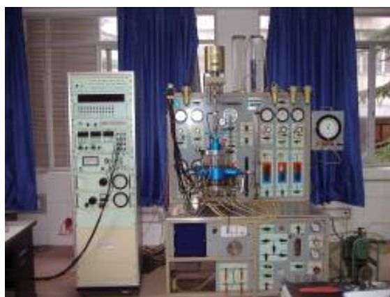
Figure 2. The 500 kN dynamic three-axis experiment system of all digital electro-hydraulic servo
