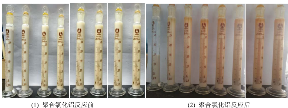
Figure 1. Comparison image of flocculation before and after the reaction of polyaluminum chloride 图 1. 聚合氯化铝反应絮凝前后对比图
