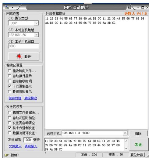
Figure 8. Transmitted data and received data of Ethernet 图 8. 以太网发送和接收数据对比图
