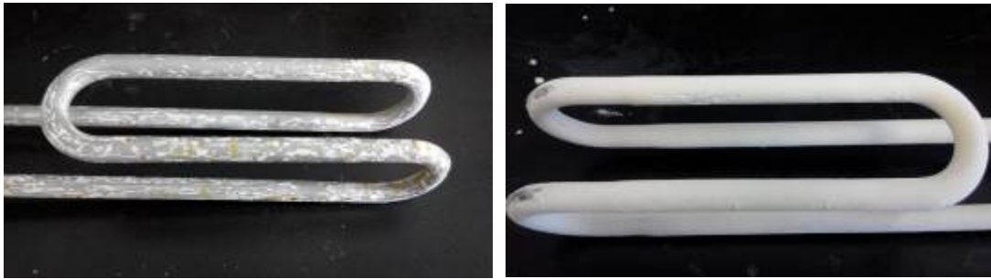
Figure 7. Surface morphology of 310S used in tap water with different \text{HCO}_3^- concentrations after 20 cycles (Left: 173 mg/L; Right: 470 mg/L)
