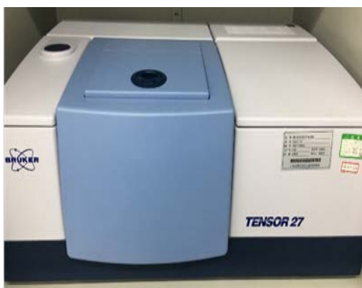
Figure 1. Bruker Fourier transform spectrometer Tensor 27 图 1. 布鲁克傅里叶红外光谱仪 Tensor 27
