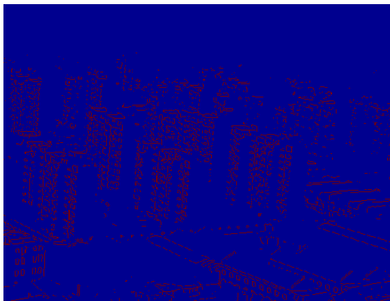
Figure 6. The image edge by Sobel algorithmic detection 图 6. Sobel 算法检测的图像边缘
