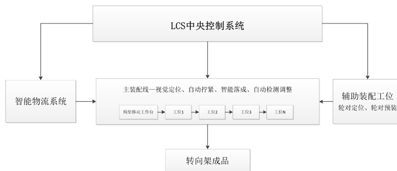
Figure 1. Process logic of the production line 图 1. 生产线工作逻辑图
