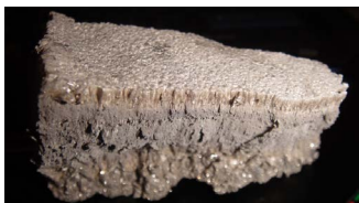
Figure 3. Condensed magnesium from reduction pot 图 3. 立式镁还原罐产生的粗镁
