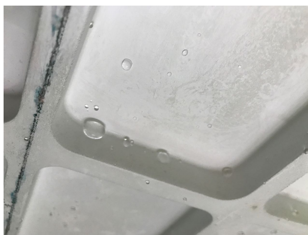
Figure 13. Hydrophobicity maintained after removing the ice 图 13. 除去冰层后依然有较好疏水性能
