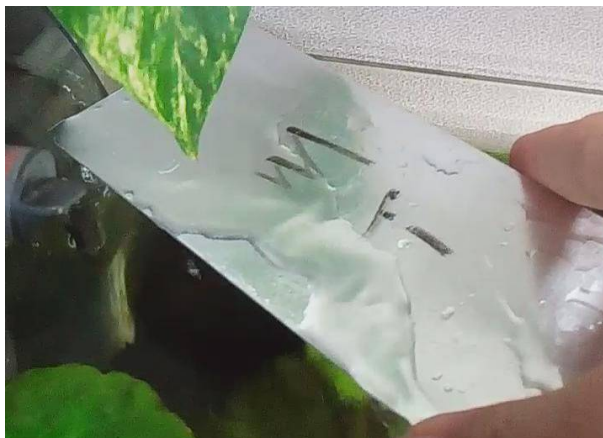
Figure 2. The uncoated test-piece exhibited hydrophilicity 图 2. 未喷涂试片表现出亲水性
