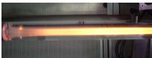
Figure 1. The fabrication process photo of fabrication of Er/Bi co-doped silica preform
